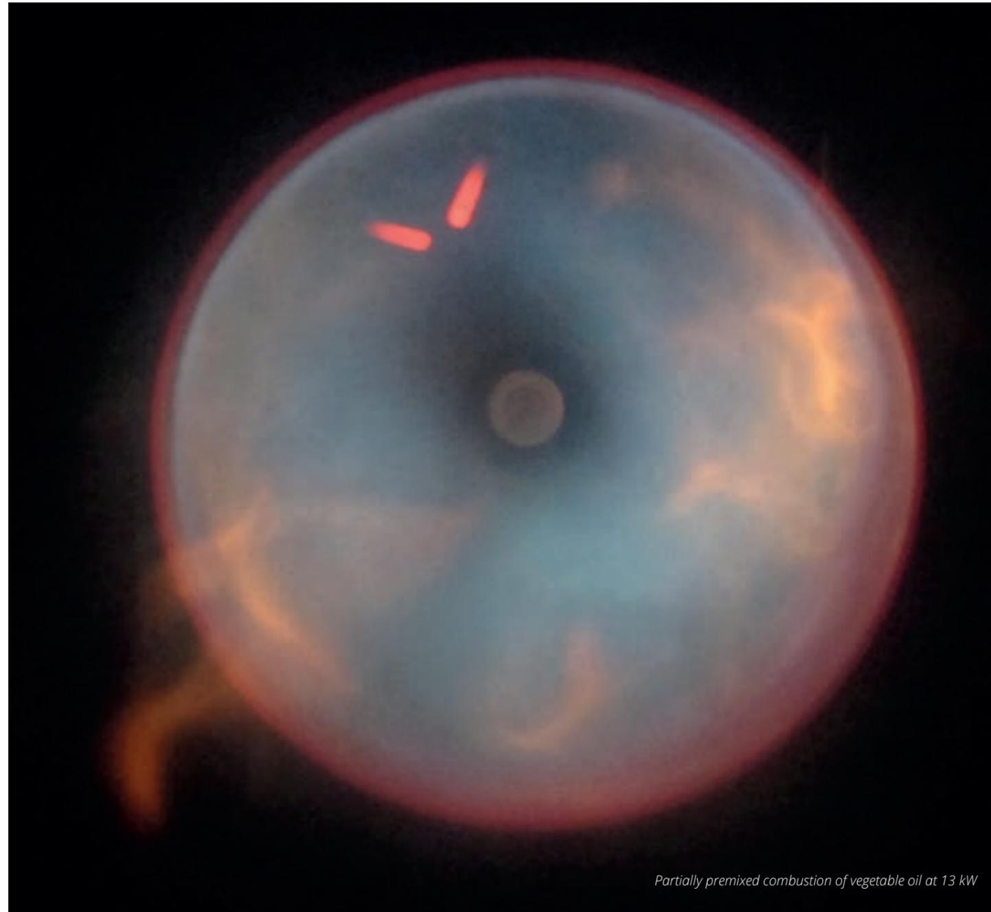
Partially premixed combustion of vegetable oil at 13 kW
